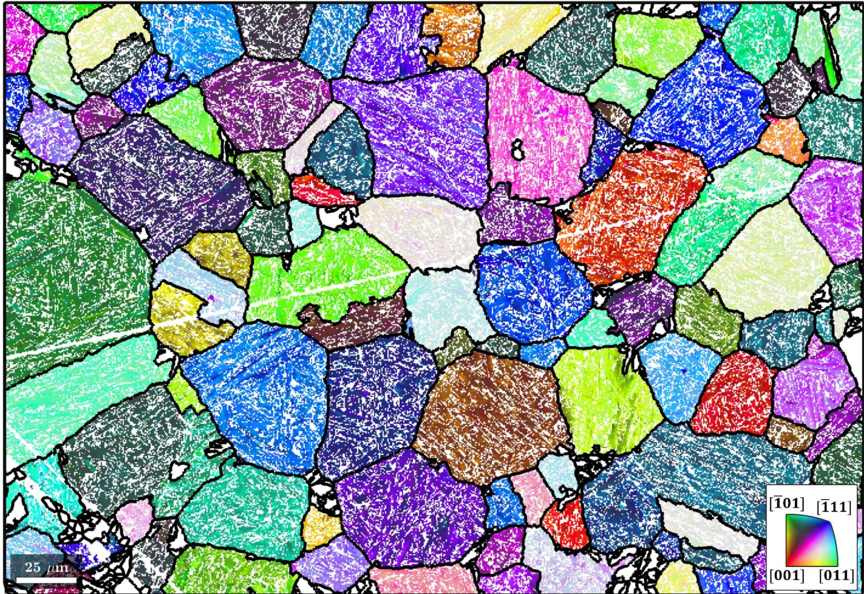
Figure 10: Reconstructed parent EBSD data with the parent grain boundaries in black.
