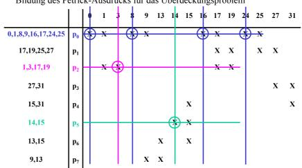
$PA = e_0(e_0 \lor e_2)e_2(e_0 \lor e_7)(e_6 \lor e_7)e_5(e_4 \lor e_5 \lor e_6)(e_0 \lor e_1 \lor e_2)$  $(e_1\vee e_2)(\underline{e_0\vee e_1})(\underline{e_1\vee e_3})(\underline{e_3\vee e_4}) \qquad \qquad \text{© Andreas K\"{o}nig Folic 4-94}$
