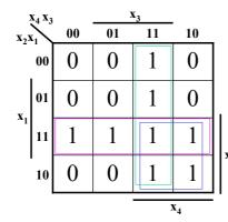
$$f_1 \wedge f_2 = x_4 x_2 \vee x_2 x_1 \vee x_4 x_3$$
