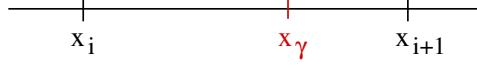
Figure 1: Graded refinement of an edge, with x_\gamma = (1 - \gamma)x_i + \gamma x_{i+1} , \gamma \in (0, 1) .
