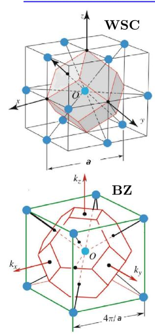
With reference to the cubic cell (a = 4.0496 Å): Wigner-Seitz cell (WSC), 1st Brillouin zone (BZ), symmetry points (SY), Fermi surface (FS)
