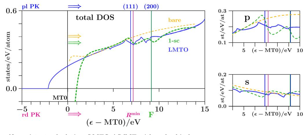
self-consistent calculation: LMTO-AS/MT with spd-orbitals interference peaks: (111),  $R^{\min}$ , and (200) at the specific free-electron energies above MTO, note the nearly perfect coincidence of (200) and F (Fermi level).
