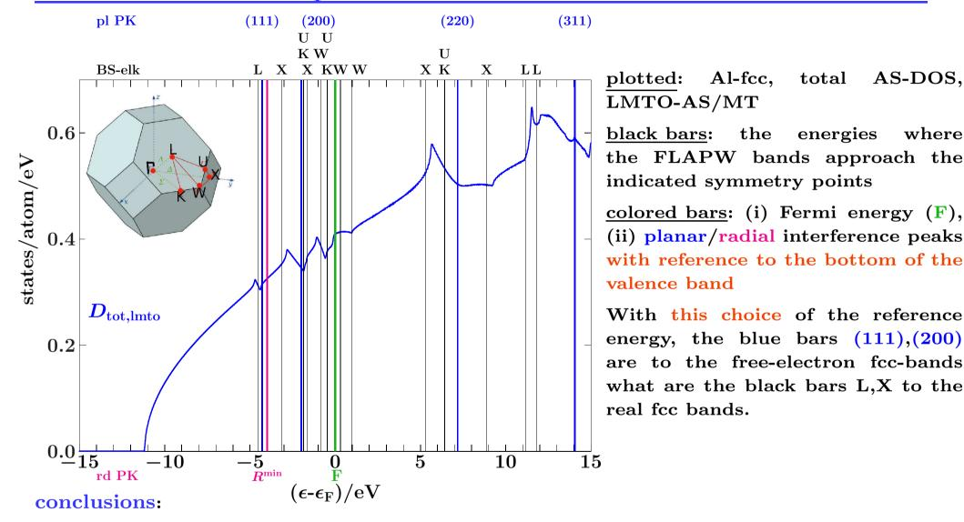
• The lowest DOS features can be assigned to symmetry point and diffraction peaks: (i) around -4.5 eV/L/(111) and (ii) around -2 eV/X/(200).
