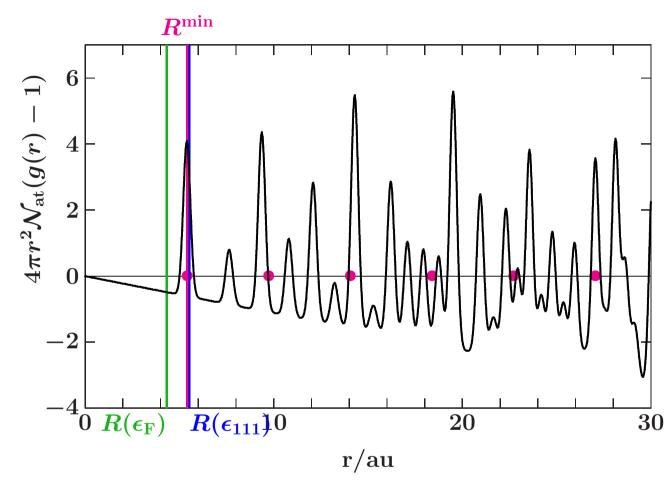
plotted: the reduced pair correlation of Al-fcc (gaussian broadening ( $\sigma \approx 0.2$  au))
