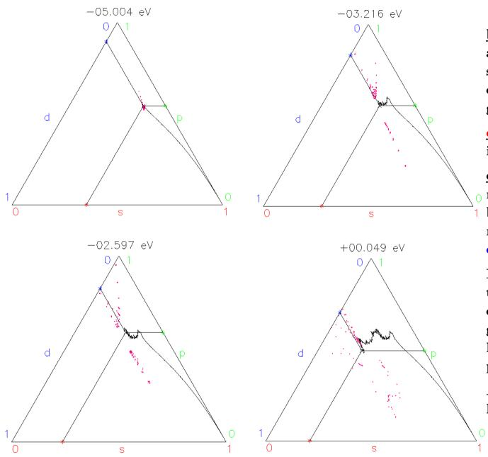
black curve: the trace of the average partial weights of band states in intervals (width 0.034 eV) around the indicated energies (s+p+d=1,  $\epsilon_F=0.0$  eV).
