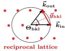
cubic lattice, side length a, planar spacing  $d_{hkl}$ , Miller indices hkl, Bragg peaks at the angles  $\Theta_{hkl}$ :
