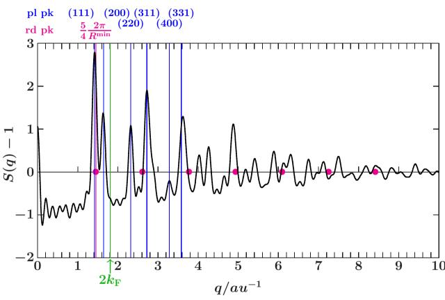
plotted: the structure factor of Alfcc as appropriate to powder diffraction (attenuation length 10 Å) top labels: the observed planar peaks, the calculated radial MDP  $dots(\bullet)$ : the expected radial diffraction peaks due to  $R^{min}$
