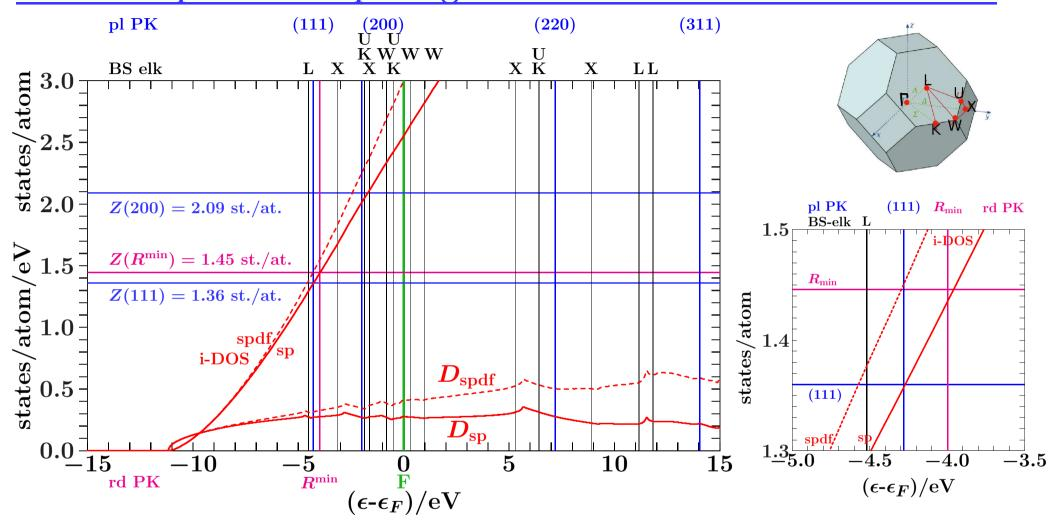
density of states  $D_{\text{spdf}}$ ,  $D_{\text{sp}}$ , integrated density of states i-DOS
