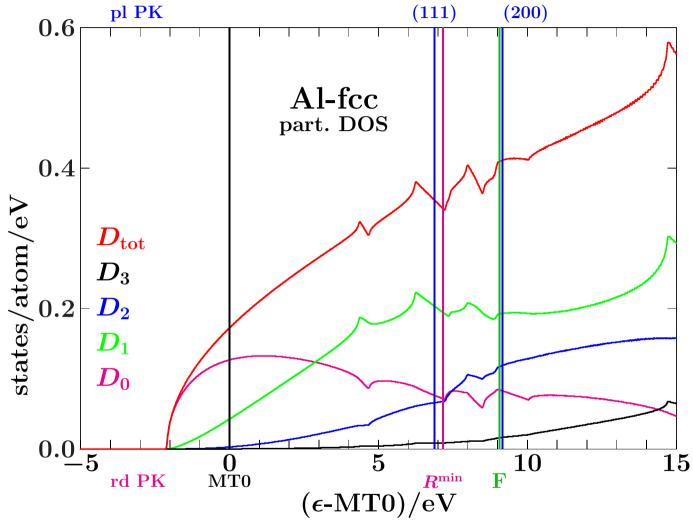
plotted: the partial DOS of Al-fcc as obtained from the LMTO-AS/MT code
