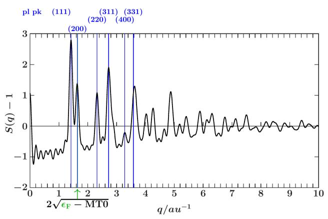
$\frac{\text{plotted:}}{\text{fcc, powder diffraction, attenuation length 10 Å}}$
